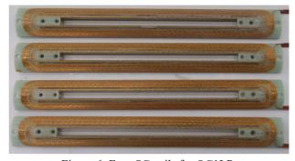
Figure 6: Four SC coils for QC1LP.
