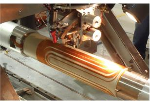
Figure 8: Winding process of corrector magnets in BNL.
