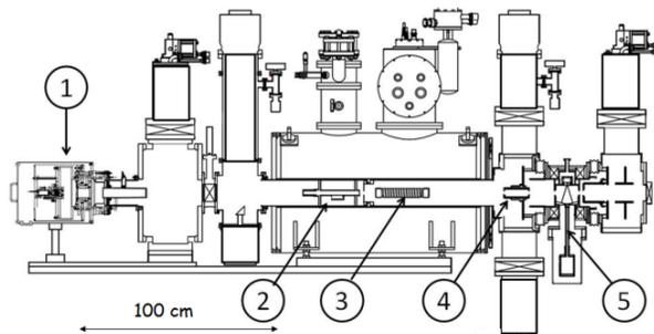
Figure 1: Layout of the OPPIS with atomic hydrogen injector: 1–high-brightness neutral hydrogen injector; 2- helium ionizer cell; 3-optically-pumped Rb cell; 4-Sona transition region; 5-sodium-jet ionizer cell.
