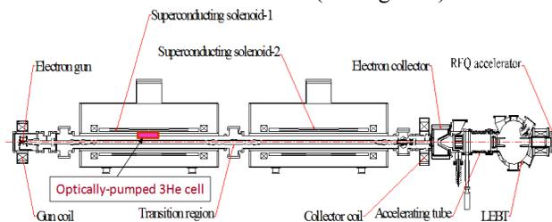
Figure 2: Schematic diagram of the extended EBIS. The polarized 3He gas is injected into the drift tube of the new “injector” EBIS part.
