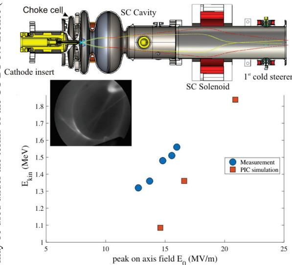
Figure 4: Measured and simulated energy gain of a field emitter located on the cathode iris opening. The inserts show a viewscreen signal of the by Solenoid focused emission area and the reconstruction by CST PIC simulation (top).
