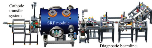
Figure 1: Overview of Gunlab housing the prototype SRF photo-injector cryo-module for bERLinPro given as picture and schematic view.
