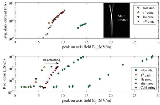
Figure 3: Average dark current measured with a Faraday Cup versus peak on axis field at the given settings. The lower plot shows the corresponding radiation level and change in field emission onset after the assembly stages and Helium processing performed after removal of the first Cu cathode.
