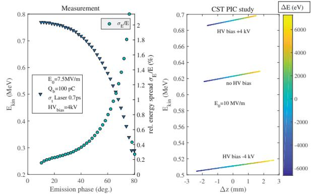
Figure 5: Measured beam energy and relative energy spread at nominally 7.5 MV/m. Reconstruction by CST PIC simulation hint at higher field level (longitudinal phase space in left column).
