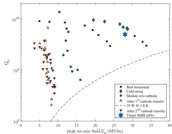
Figure 2: Intrinsic quality factor measured at each assembly or commissioning stage versus peak on axis field of the  $TM_{010}-\pi$  mode. All data sets except the first were measured by Helium boil off rate.
