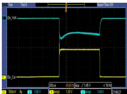
Figure 1: The magnetron arc-discharge operation. The yellow trace is the 14 A discharge current, the blue trace is the 150 V arc-discharge voltage.
