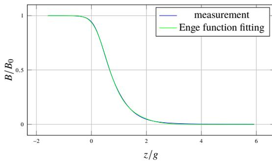
Figure 5: Typical fringe field profile of the 90-mm gap dipole along the  $z$  direction where  $z=0$  is at the pole face and  $g$  is the pole gap size.
