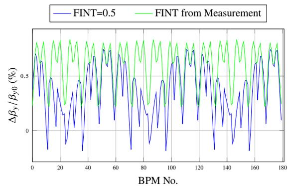
Figure 7: Deviations in the vertical  $\beta$  values from the hard-edge design values depending on the dipole fringe field effects.
