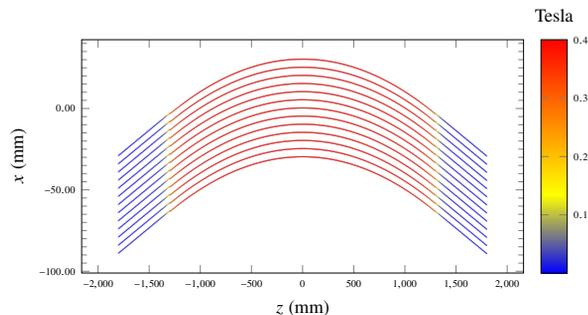
Figure 3: Hall-probe field measurement data of a sampled NSLS-II 35-mm gap dipole at  $y = 0$ .
