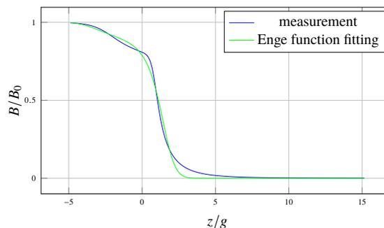
Figure 4: Typical fringe field profile of the 35-mm gap dipole along the  $z$  direction where  $z=0$  is at the pole face and  $g$  is the pole gap size.
