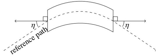
Figure 2: Schematic diagram of the rectangular dipole magnet and the ideal beam path.
