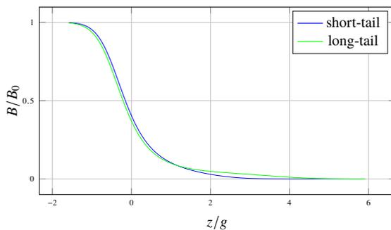
Figure 6: Typical short-tail and long-tail fringe field profiles.
