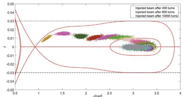
Figure 4: Beam injected at  $dt=-2ns$  away from the circular bunch and passed through over 10000 turns.
