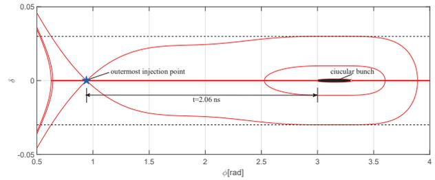
Figure 1: The main bucket formed by the triple-frequency RF system. Blue star points present the outermost injection point, black filled ellipse present the circular bunch in the main ring.
