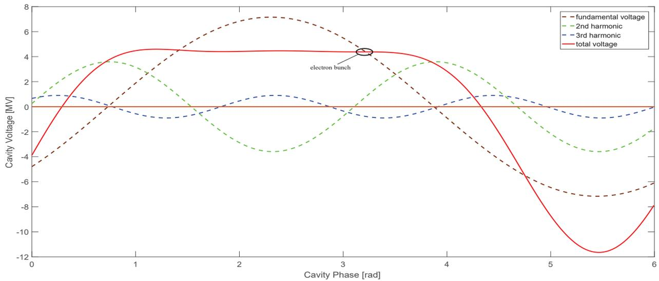
Figure 2: RF voltage seen by the bunch for the triple-frequency RF system.
