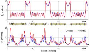
Figure 3:  $\beta_x$  (top) and  $\beta_y$  (bottom) are plotted as blue curves for the design and red curves for the measurement at the 100 MeV operation mode.
