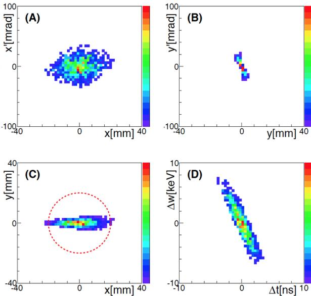
Figure 2: Simulated phase space distributions at the MCP detector. (A) the horizontal divergence angle  $x'$  vs the horizontal position  $x$ , (B) the vertical divergence angle  $y'$  vs vertical position  $y$ , (C)  $y$  vs  $x$ , and (D) the displacement from the mean kinetic energy  $\Delta w$  vs the displacement from the mean TOF  $\Delta t$ . Red dotted line shows the effective area of the MCP detector.
