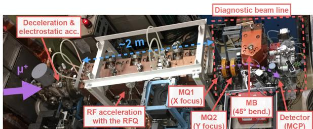
Figure 1: Experimental setup of the muon acceleration test.
