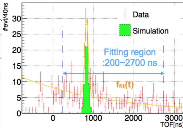
Figure 3: MCP timing distribution when the RF was on and the threshold was 200 mV.
