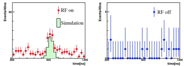
Figure 4: Comparison of MCP timing distributions between the RF-on and RF-off data, and simulation. The numbers of triggers for RF-on and RF-off data are  $4 \times 10^6$  and  $4 \times 10^5$ , respectively.
