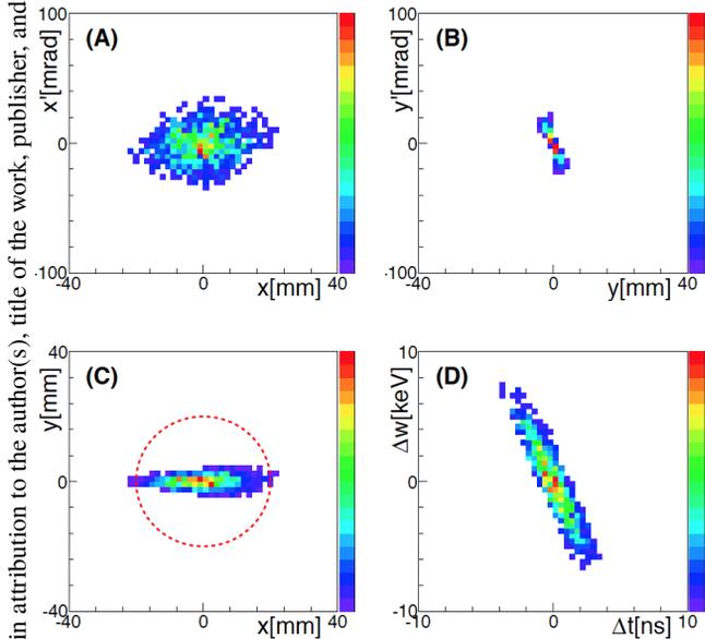
Figure 2: Simulated phase space distributions at the MCP detector. (A) the horizontal divergence angle  $x'$  vs the horizontal position  $x$ , (B) the vertical divergence angle  $y'$  vs vertical position  $y$ , (C)  $y$  vs  $x$ , and (D) the displacement from the mean kinetic energy  $\Delta w$  vs the displacement from the mean TOF  $\Delta t$ . Red dotted line shows the effective area of the MCP detector.
