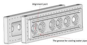
Figure 3: Schematic drawing of the tank half shells.
