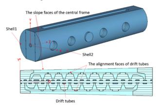
Figure 4: A CST model of IH-DTL for error analysis.
