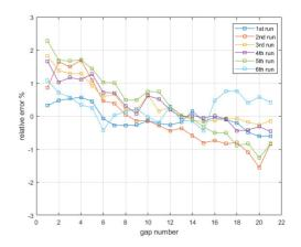
Figure 6: Calculated relative error of gap voltage distribution for different error setting.
