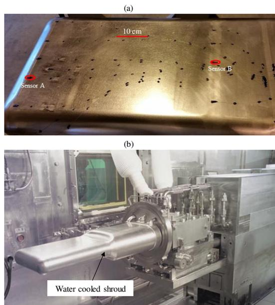
Figure 2: (a) Sensors mounted on the mercury target vessel. Strain measurement results from sensors A and B will be described. (b) Target module (mirrored image) mounted on target carriage in the target service bay. The target vessel is covered by water cooled shroud during operation.
