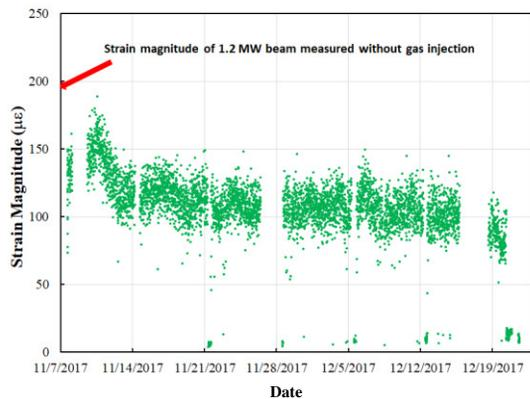
Figure 4: Strain magnitudes of 1.2 MW neutron production beam measured from sensors B on SNS target T18 with gas injection. The reference level indicates the strain magnitude of the 1.2 MW beam measured without gas injection.
