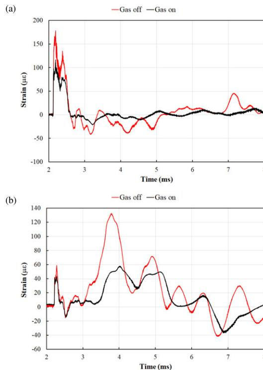
Figure 3: Strain waveforms measured with sensor A (a) and sensor B (b) at gas injection off and on. The proton beam power is 1.2 MW (equivalent) in both cases.
