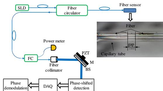
Figure 1: Schematic of fiber-optic strain sensor. SLD: superluminescent laser diode, PD: photo-detector, FC: fiber coupler, M: mirror, BS: 50/50 beam splitter, PZT: piezoelectric transducer actuator, DAQ: data acquisition unit. Inset box: microscopic image of sensor head.
