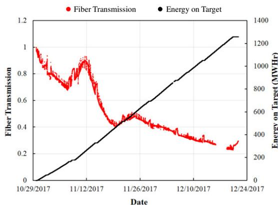
Figure 5: Normalized fiber transmission of sensor B and proton beam energy delivered on the SNS target T18.
