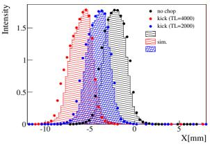
Figure 3: Beam profiles in the horizontal direction. The black, the red, and the blue dots show the measurements by the WSM for several field strengths of the RFD. The black, the red, and the blue histrograms show the simulations.
