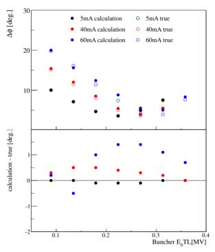
Figure 4: Results of virtual measurements using the simulations. (Top) the calculated longitudinal width, and (bottom) the differences between the calculations and the true values.
