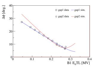
Figure 5: Result of measurement of the longitudinal bunch size using the first gap of the RFD (square) and second gap (circle). The blue and the red lines show the simulations after fitting the measurements for the first gap and the second gap, respectively.
