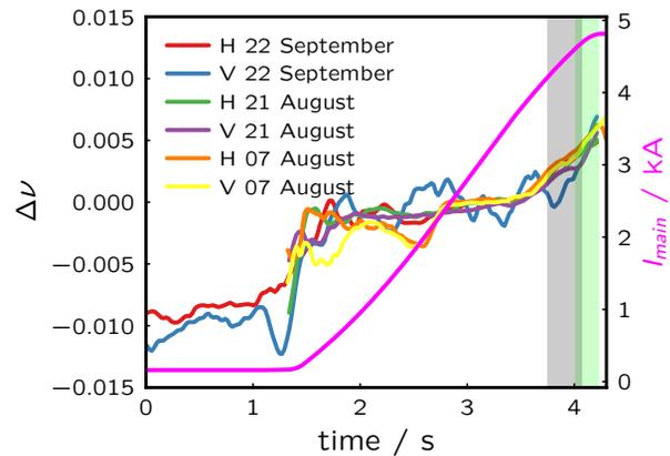
Figure 3: Difference of horizontal and vertical tune along FT cycle before and after a SC change. The magenta line represents the current time evolution of the main SPS PS.
