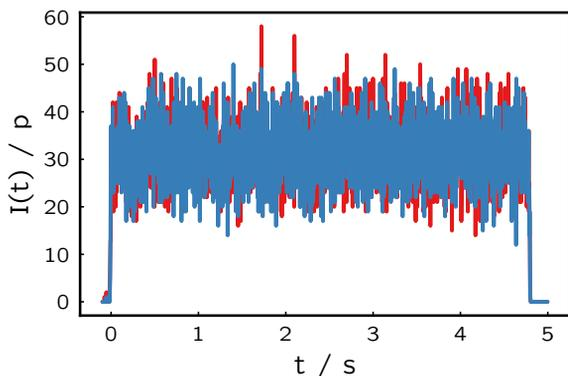
Figure 6: Example of spill structure simulations using the described semi-analytic model. In red, the expected spill structure when 50, 100 and 150 Hz noise on the horizontal tune is injected. In blue, the same noise is used, but the extraction speed was increased by 50 %, together with the extraction sextupole strength.
