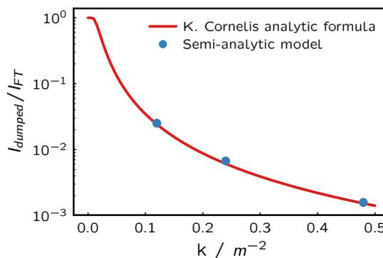
Figure 7: Evolution of non-extracted particles, normalised by the total intensity, as a function of the sextupole strength. In red, the analytic formula presented in [10] is shown. The blue markers represents the results obtained with the described semi-analytic model.
