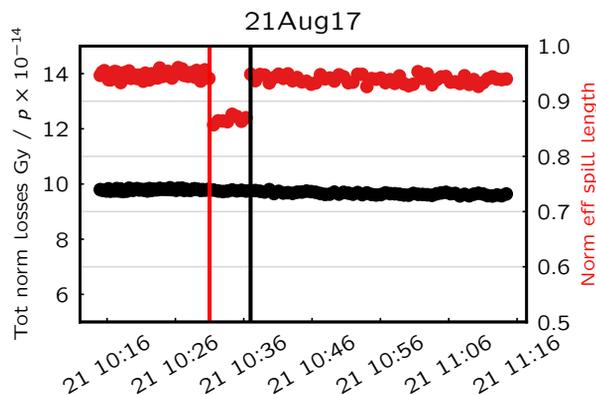
Figure 1: Time evolution of normalised effective spill length and total extraction losses in the slow extraction channel. The vertical red line represents a change in SC and the black vertical line the correction applied on the tune to readjust the spill quality.
