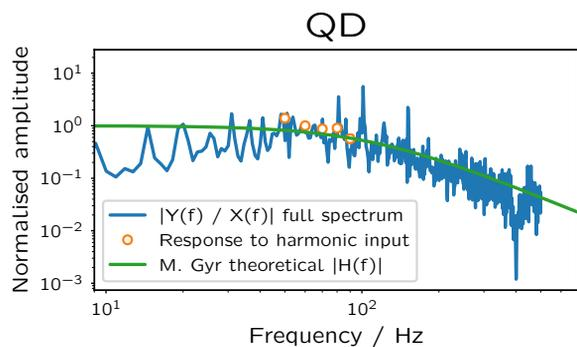
Figure 5: Transfer function between QD PS and extracted intensity.
