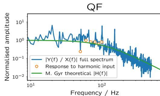
Figure 4: Transfer function between QF PS and extracted intensity.
