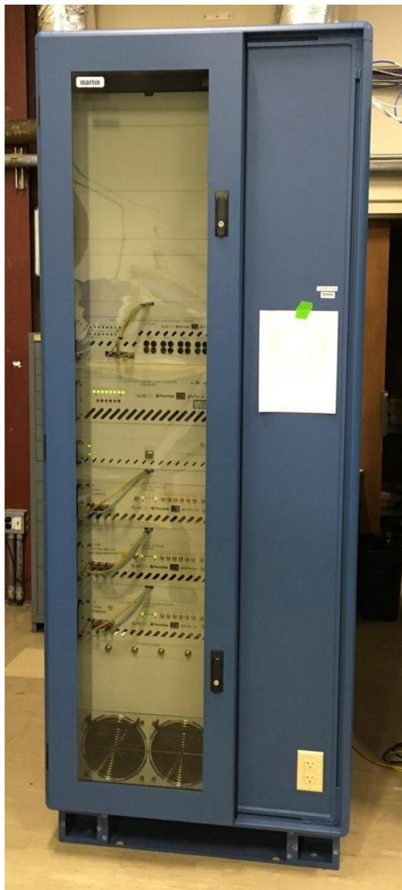
Figure 4: Fully integrated LLRF rack at the SLAC test stand.
