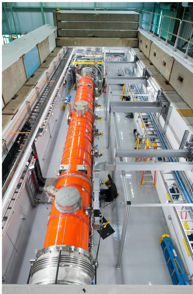
Figure 3: Cryomodule at the Fermilab CMTF (courtesy of FNAL).
