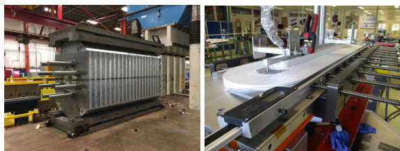
Figure 9: The US 15 T magnet prototype at FNAL (left) and a 16 T enhanced racetrack coil at CERN (right).
