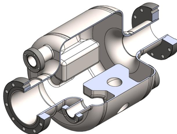
Figure 1: The SRF deflecting cavity geometry showing the fabrication of the ridges from solid niobium with a cooling channel to allow cooling from the inside of the ridge.
