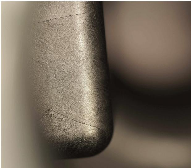
Figure 3: The surface appearance of the ridge showing the pitting after the 120  $\mu\text{m}$  etch.
