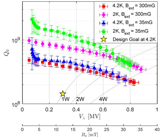
Figure 4: The cavity performance measured in ambient magnetic fields of 300 and 35 mG.
