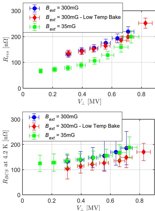
Figure 5: The field dependence of the residual resistance (top) and BCS resistance at 4.2 K (bottom), extracted from the surface resistance data.
