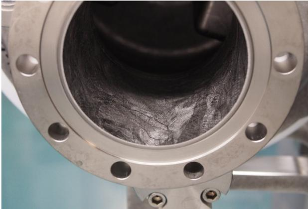
Figure 2: The surface appearance of the upstream beam pipe after the 120  $\mu\text{m}$  etch.
