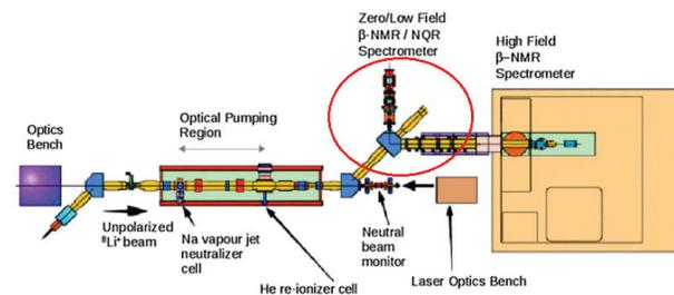
Figure 2: Present  $\beta$ -NMR beamline with two spectrometers covering different magnetic field ranges [6]. The low-field spectrometer section (circled in red) is the location for the upcoming  $\beta$ -SRF extension facility.
