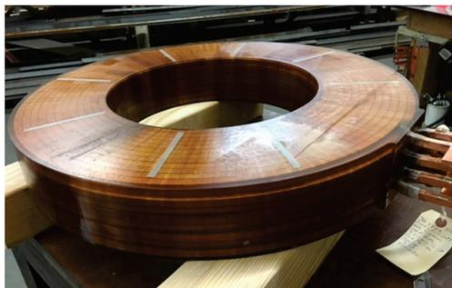
Figure 4: Photo of Helmholtz coil operated at 200 mT which has been recently received at TRIUMF.
