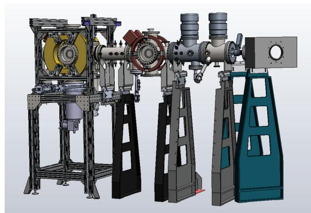
Figure 3: Mechanical design of the extended  $\beta$ -NMR beamline for  $\beta$ -SRF facility. The added stronger Helmholtz coil is shown in the far left (gold colour) coil together with its support frame.
