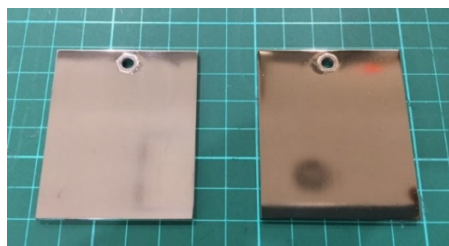
Figure 6: Electro polished Nb bare substrate (the left) and NbN/SiO 2 deposited Nb substrate (the right).
