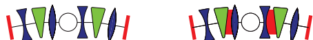
Figure 1: Left: Standard section with 4 quads (blue), 2 dipoles (green), and 1 vertical corrector (red). Right: Extra corrector section with 2 extra vertical correctors put in.
