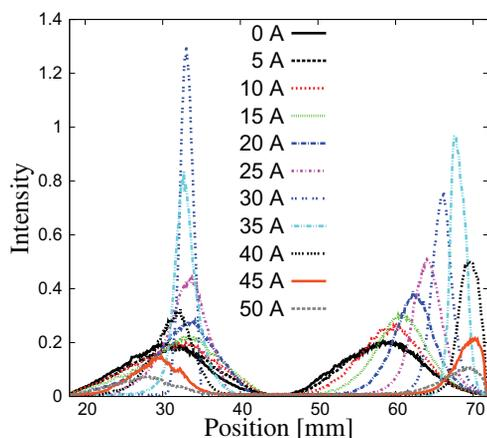
Figure 2: Effect of mis-aligned solenoid at various currents.
