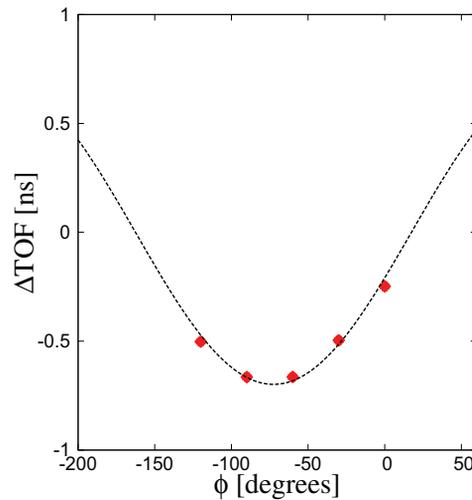
Figure 1: Cosine fit of Cavity TOF vs Phase Data.
