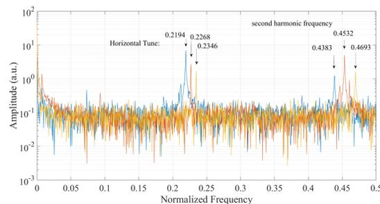
Figure 5: Size spectrum comparison of maximum amplitude bunch in three injections.
