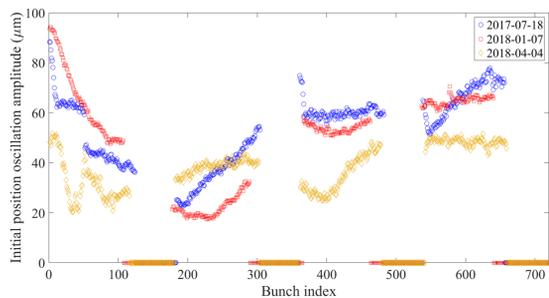
Figure 1: Initial position oscillation amplitude distribution in bunches of three injections.
