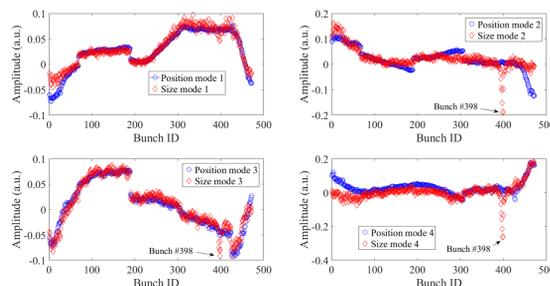
Figure 8: First 4 modes waves comparison of bunch-by-bunch position and size distributions after PCA analysis.
