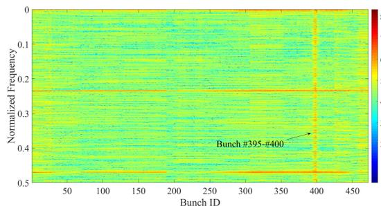
Figure 9: Spectrum waterfall plot of turn-by-turn size oscillation.
