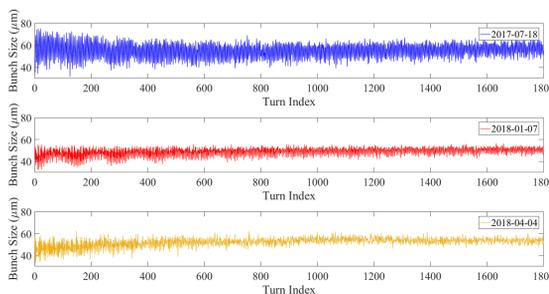
Figure 3: Size temporal wave comparison of maximum amplitude bunch in three injections.
