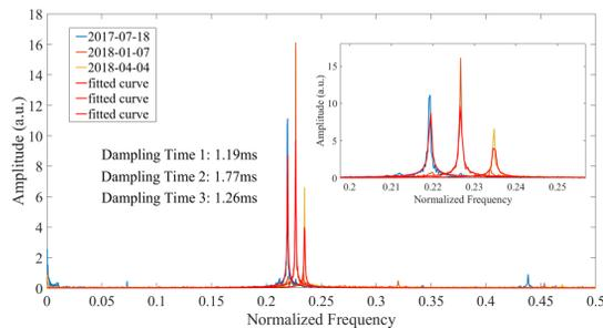
Figure 6: Damping time fitting results in three injections.
