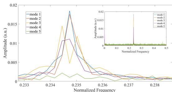
Figure 7: PCA modes spectrums of turn-by-turn position oscillation.
