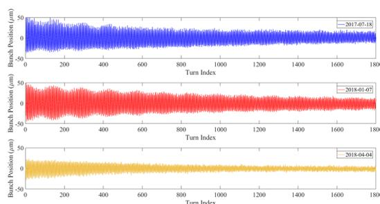
Figure 2: Position temporal wave comparison of maximum amplitude bunch in three injections.
