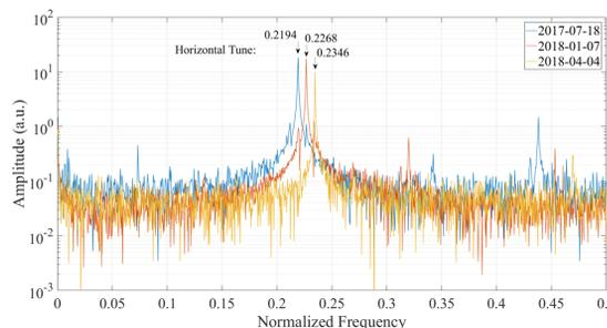
Figure 4: Position spectrum comparison of maximum amplitude bunch in three injections.
