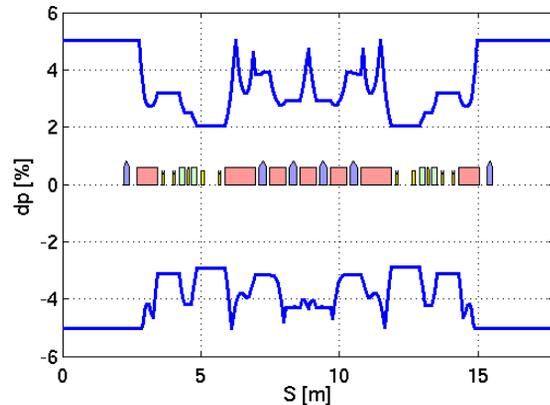
Figure 4: Touschek relative energy acceptance along a single cell.
