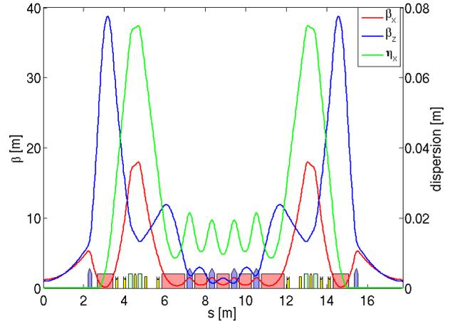
Figure 1: Optical function of the SOLEIL baseline lattice.
