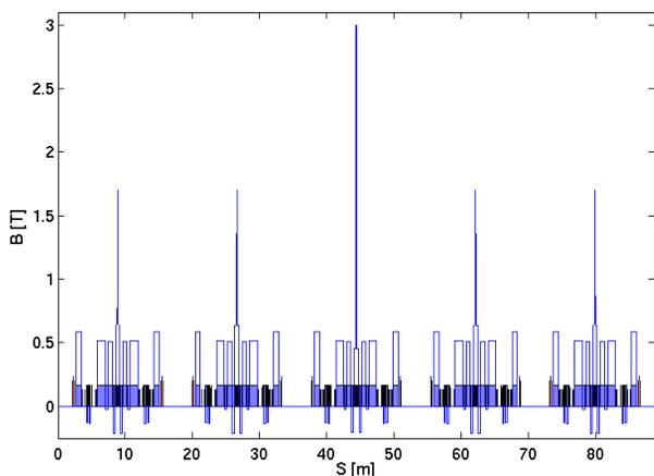
Figure 6: Dipolar magnetic field profile along 5 cells of the upgraded lattice with peak fields of 1.8 and 3 T.
