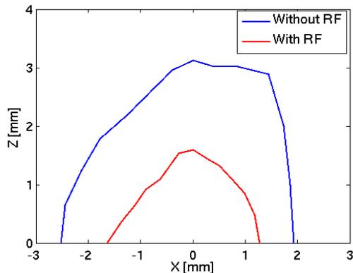
Figure 2: On-momentum dynamic aperture at straight center section with  $\beta_x=1.3$  and  $\beta_z=1.0$  m.rad<sup>-1</sup>.
