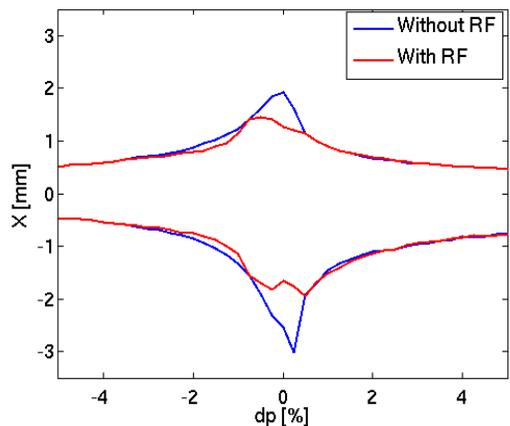
Figure 3: Horizontal dynamic aperture versus energy deviation at straight section center with  $\beta_x=1.3$  m.rad<sup>-1</sup>.
