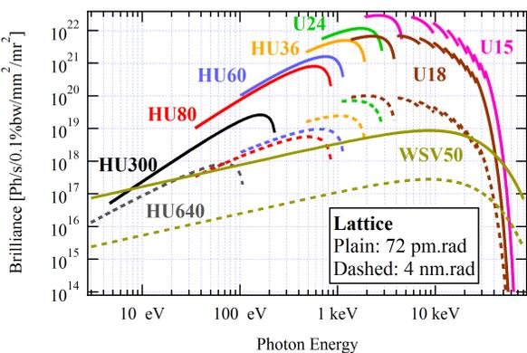
Figure 6: Photon beam brilliance comparison of between upgraded and present SOLEIL storage ring.
