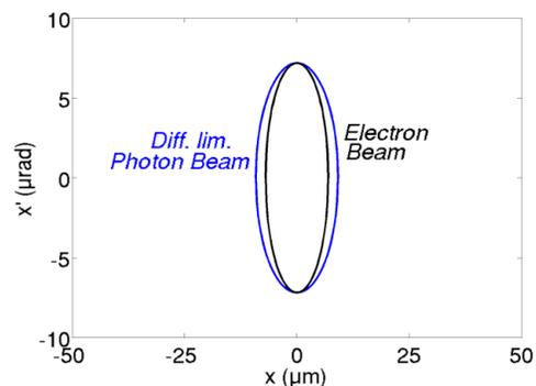
Figure 5: Matched phase space between the 50 pm.rad electron beam and the 65 pm.rad photon (3 keV) beam over 4 m long undulator.
