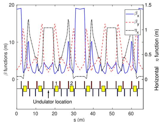
Figure 2: The nominal HLS-II lattice with an undulator inserted for laser bunch slicing.
