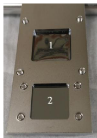
Figure 5: Two RTR emitters mounted on a fixture. Emitter #1 is 100 periods Mo/Si deposited on a kapton foil and emitter #2 is the same structure deposited on a 100 \mu\text{m} Si substrate.
