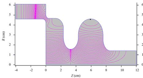
Figure 4:  $\pi$  mode electric field distribution of the RF gun after optimization (Unit: cm).
