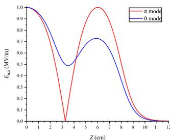
Figure 5: Longitudinal electric field of the  $\pi$  mode and 0 mode.
