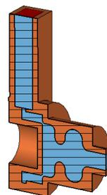
Figure 1: Cross section of the proposed rotationally symmetric RF gun.
