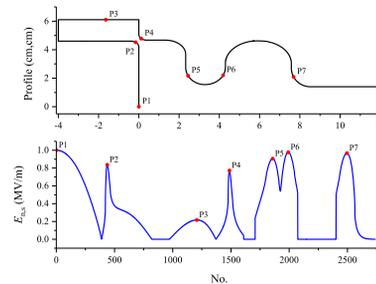
Figure 7: Surface electric field along the inner cavity.
