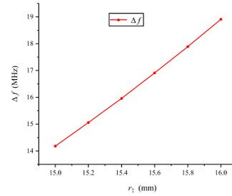
Figure 6: Mode separation vary with the iris diameter.
