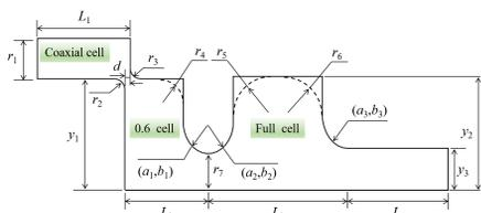
Figure 3: Cross section of the 1.6 cell RF gun. (Solid line is the original gun; Dash line is the optimized gun.)
