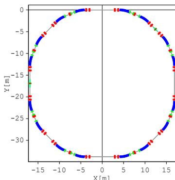
Figure 1: Model of the KARA ring [2]. The  $22.5^\circ$  bending magnets are depicted in blue, quadrupoles in red and the sextupoles are marked in green. The CATACT/CLIC wigglers are shown by long green strips. Octupole components of wigglers are represented by brown strips in the middle of insertion device.
