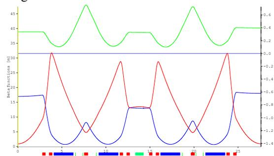
Figure 2: One cell of the KARA lattice is composed of two pairs of  $22.5^\circ$  bends. The middle of long straight section where the CLIC wiggler is located is chosen as an origin ( $\theta_0=0$ ). The horizontal/vertical beta-functions are depicted in blue/red dispersion – green.
