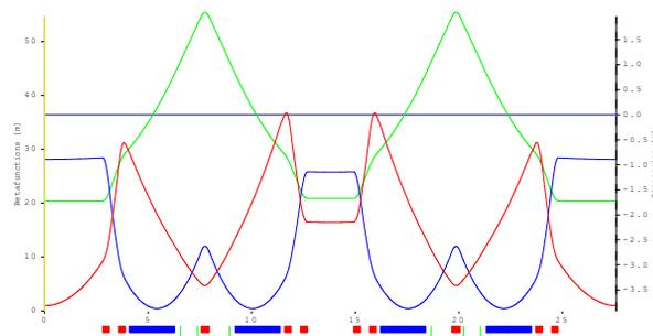
Figure 3: KARA lattice at low-alpha operation mode. Span of dispersion is increased to  $\pm 1.8$  m in order to compensate positive and negative contribution of dispersion inside bending magnets. Compaction factor at low- $\alpha$  was reduced down to  $5 \cdot 10^{-5} \div 10^{-4}$ .
