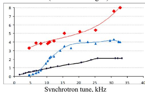
Figure 9: Life time (vertical axes - in hours) as function of synchrotron tune. Black curve - simulations, Blue curve - measured data before sextupole corrections, red curve - after corrections.
