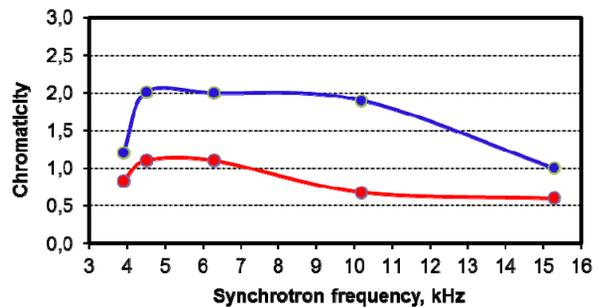
Figure 8: Optimized horizontal (blue) and vertical (red) chromaticity measured during low alpha squeeze.
