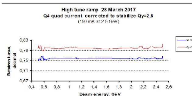
Figure 7: High tune ramp corrected to keep tune unchanged. Red curve is horizontal tune, blue curve is vertical tune.
