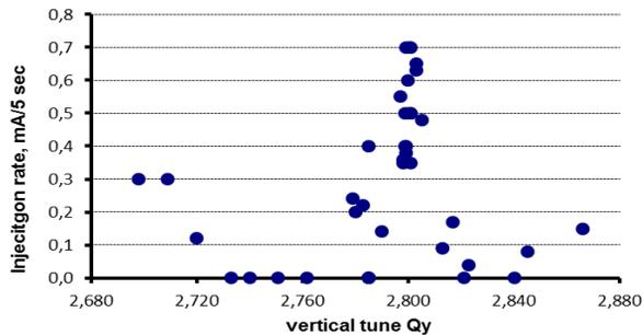
Figure 5: Injection rate of KARA beam at high vertical tune. The best injection conditions correspond to tune  $Q_y=2.801$ .
