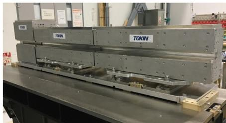
Figure 1: Permanent magnet based longitudinal gradient bending magnet. The total length is about 1.7 meter.
