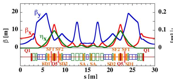
Figure 1: Lattice functions of SPring-8-II.
