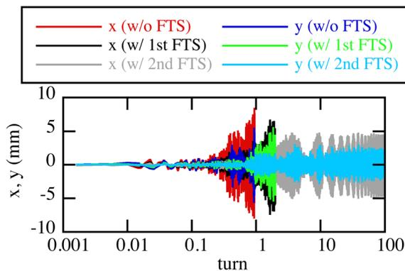
Figure 2: Trajectory of injected beam.
