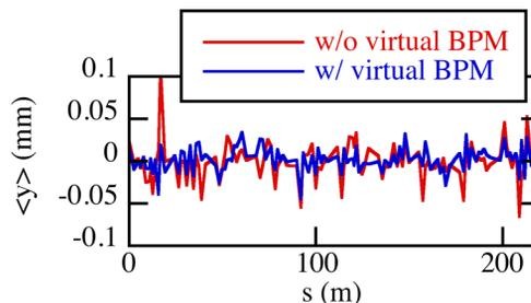
Figure 9: COD after correcting with virtual BPM.
