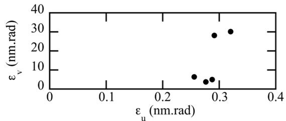
Figure 7: Emittance growth in the vertical due to misalignment of quadrupoles.
