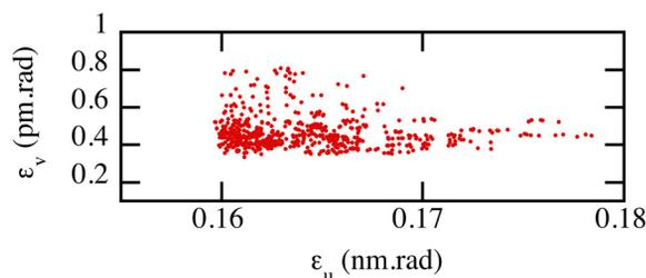
Figure 4: Emittance with machine imperfections.
