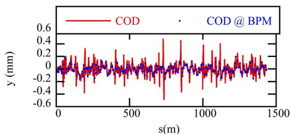
Figure 8: Continuous COD and sampled one by BPM.
