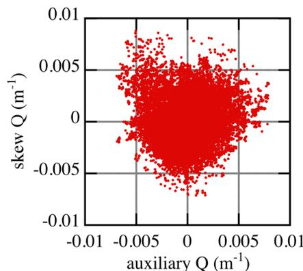
Figure 5: The auxiliary and the skew quadrupole fields.
