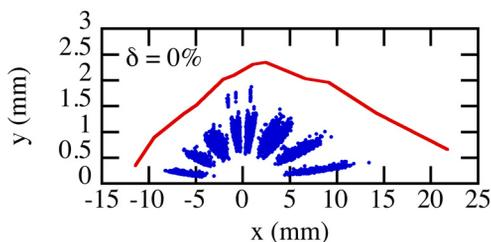
Figure 3: On-momentum DA (red) without error and (blue) with machine imperfections after FTS method.
