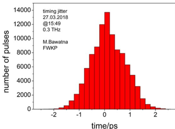
Figure 5: Measured timing jitter of the THz pulses.
