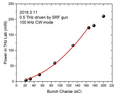
Figure 2: Measured THz power vs. bunch charge.
