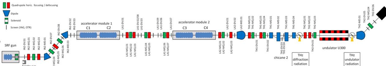
Figure 1: ELBE accelerator beamlines for THz radiation production with the SRF Gun II.
