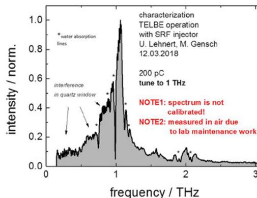
Figure 3: THz spectrum for 1 THz tuning.
