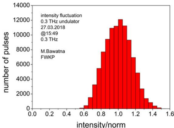
Figure 4: Measured intensity fluctuations of the THz pulse energy for 0.3 THz.
