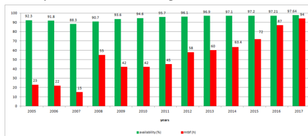
Figure 1: Combined graph of Elettra availability (in %, green bars) and MTBF (in hours, red bars).
