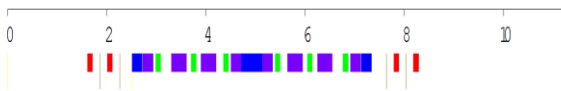
Figure 7: Magnet arrangement from centre of mid straight section to middle of standard straight section in 6RB-BA lattice. The blue, purple, red and green colours indicate to longitudinal, transverse dipoles (including anti-bend), quadrupole and sextupole magnets respectively.
