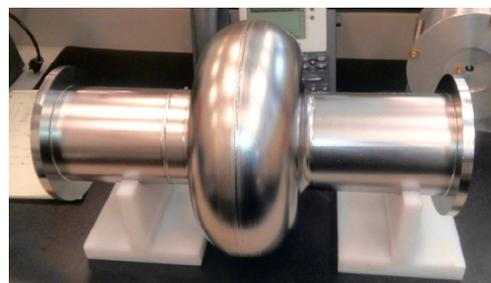
Figure 7: First 952.6 MHz cavity at JLab.
