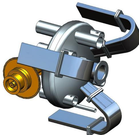
Figure 1: On-cell damper storage ring cavity concept.
