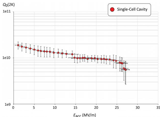
Figure 8: Preliminary Result of 952.6 MHz 1-cell cavity.
