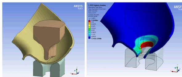
Figure 9: Simulation of on-cell damper iris formation.
