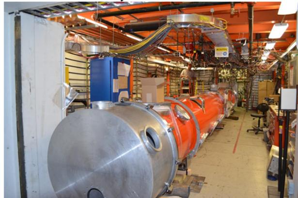
Figure 2: LCLS II Cryomodule in Test Cave
