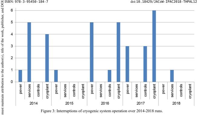
Figure 3: Interruptions of cryogenic system operation over 2014-2018 runs.
