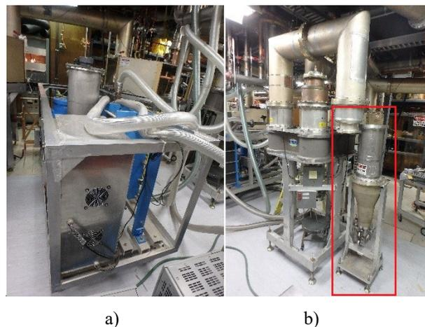
Figure 3: The 600 kW sodium bicarbonate filled Dummy Load with in the RF Room.
