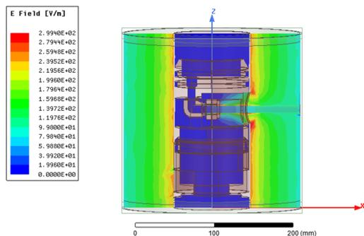
Figure 9: The simulation of water feedthrough.
