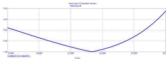
Figure 2: VSWR of the Dummy Load.
