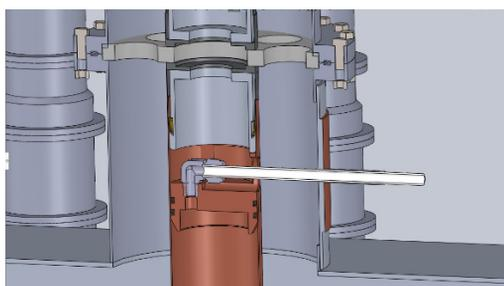
Figure 7: Water Feedthrough at the Entrance of the 1.1 MW Dummy Load.
