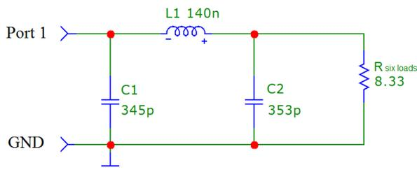
Figure 1: The Schematics of 1.1 MW Dummy Load.
