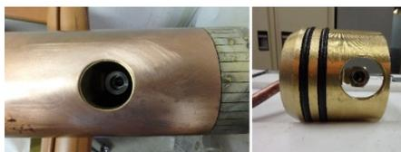
Figure 8: Water bullets used in the 9-inch transmission line for water feeding.
