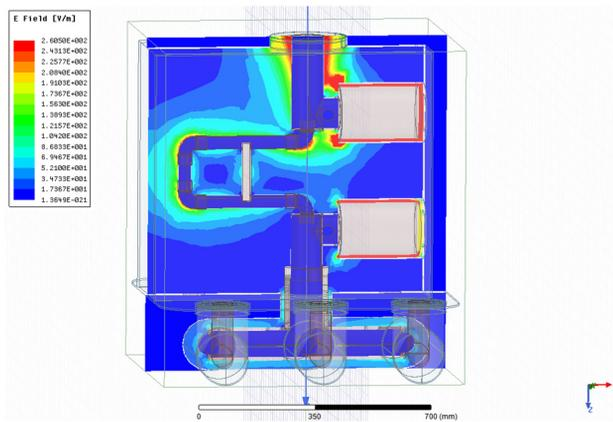
Figure 5: The distribution of the electric field in RF field's the middle plane (result of simulation in HFSS)
