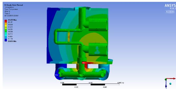
Figure 6: Temperature distribution calculated by ANSYS Workbench.
