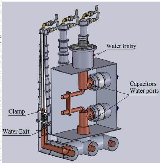
Figure 4: The Design of 1.1 MW Dummy Load.
