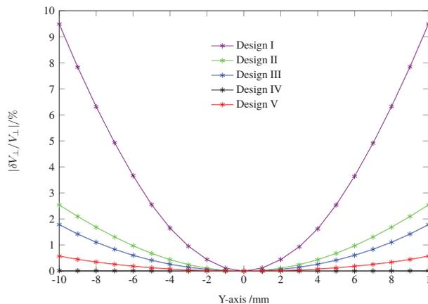
Figure 5: Relative transverse voltage variation along the y-axis for all the five cavity designs.
