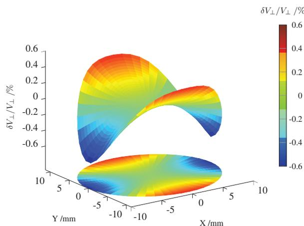
Figure 4: The relative transverse voltage variation in the circular region of radius 10 mm around the axis of the cavity for Design-V. The beam transverse along the z-axis.
