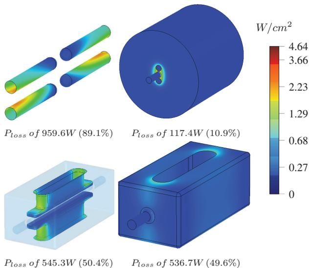
Figure 3: Distribution of the surface power loss on the inner (left) and outer part (right) of the cavity for Design-I (top) and V (bottom).
