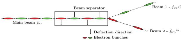
Figure 1: Sketch representing the working principle of a beam separator.
