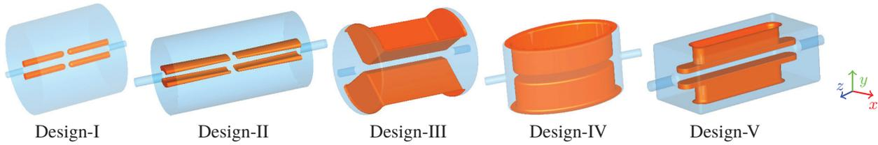
Figure 2: Geometry of the five probable deflecting cavity designs: CEBAF deflector (Design-I), probable crab cavities of LHC (Design-II,III,IV) and a novel NC deflecting cavity (Design- V). The outer surfaces of the cavity are made transparent to highlight the inner parts. The beam traverses along the  $z$ -axis.
