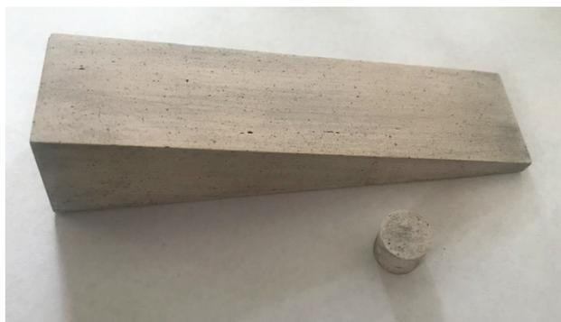
Figure 5: 90-92% dense ceramic with surface pores filled with sub-micron carbon particles.
