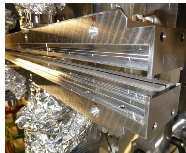
Figure 3: 1 m passive device (gap in the vertical plane) which will be installed at the SwissFEL injector. Two over the three corrugations are also visible.
