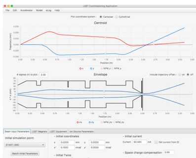
Figure 1: LEBT application GUI interface. On the top the Menu Bar is created from the FxApplication class. The plots show the trajectory (top chart) and envelope (bottom chart) together with NPM readings. On the bottom of the application panel there are 4 tabs: beam input parameters, input values for the LEBT magnets, LEBT diagnostics display and input values for Ion Source magnets and power supplies.
