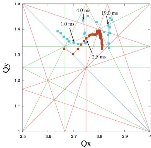
Figure 5: MAIN RING betatron tune footprints. Blue and brown squares indicate measurements and simulations, respectively.
