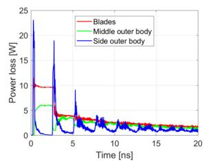
Figure 6: Energy dissipated on the blades during and after the bunch passage.
