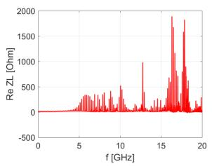
Figure 3: The real part of the longitudinal impedance.
