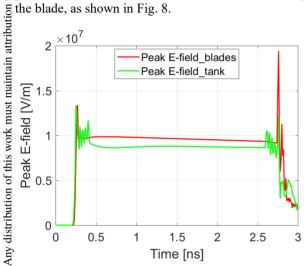
Figure 7: Maximum electric field on the blade and on the 8). outer body. The red curves presents the peak electric field 201 on the kicker blades and the green curve shows the peak Q electric field on the outer body.
