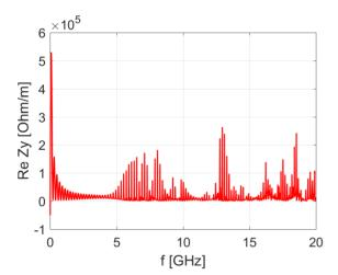
Figure 4: The real part of the transverse impedance.
