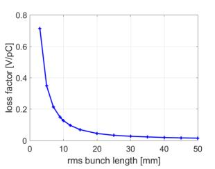
Figure 5: Dependence of the longitudinal loss factor on the rms bunch length.
