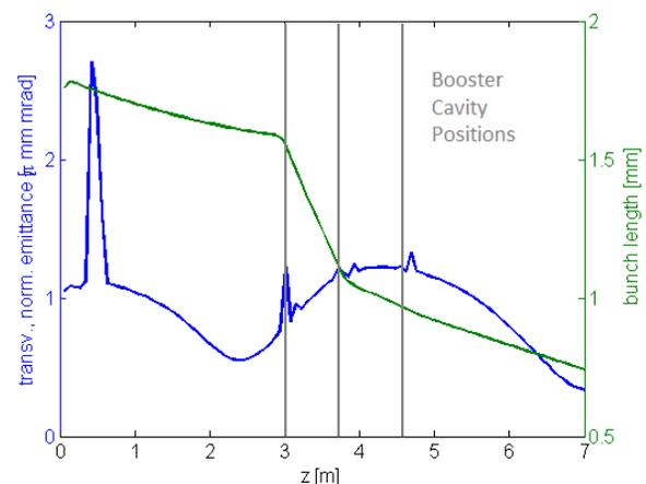
Figure 3: Evolution of the transverse emittance (blue) and bunch length (green) along the beam axis for the high-brightness setting in Fig. 2.
