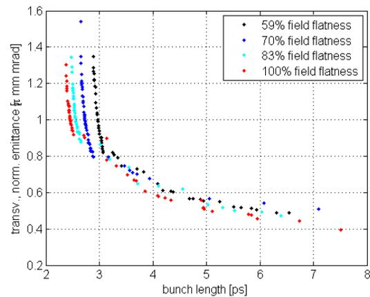
Figure 4: Pareto curves for 100% field flatness (red) and for field enhancement in the gun cavity full-cell.
