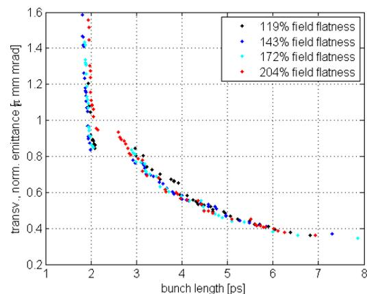
Figure 5: Pareto curves for field enhancement in the gun cavity half-cell.
