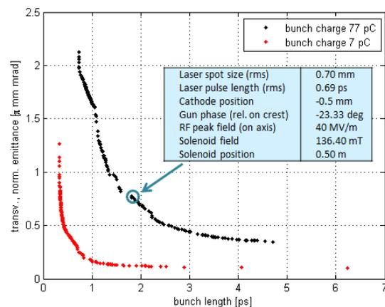
Figure 1: Pareto optimum curves for 7 pC (diagnostic mode) and 77 pC (high average current mode) of the bERLinPro SRF photoinjector.
