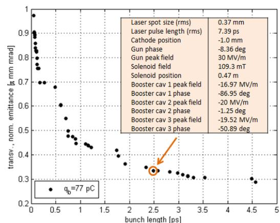
Figure 2: Pareto optimum settings for an SRF photoinjector followed by a 3 cavity booster section (bERLinPro design) for high brightness operation.
