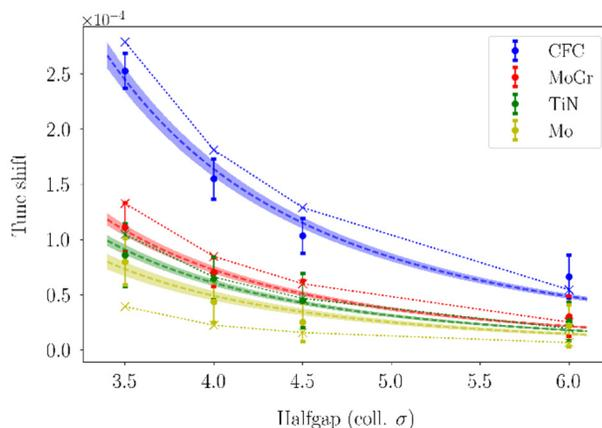
Figure 5: The use of MoGr (red) reduces the resistive wall tune shift compared to the uncoated CFC (blue); each type of coating: TiN (green) and Mo (yellow) further improves the conductivity and can be clearly differentiated. For most materials the results (dots show the measured data and dashed curves – its fits with their  $\pm 1$  rms uncertainties) are within 10-20 % of the model predictions (dotted lines).
