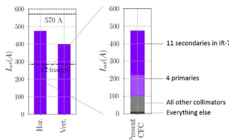
Figure 1: Impedance of LHC collimators is responsible for nearly all the octupole current needed to stabilize the beam, and has to be reduced to provide a stability margin for the Hi-Lumi upgrade [3]. BCMS beam, 7 TeV, beginning of the luminosity levelling process,  $\beta^* = 41\ \text{cm}$ .
