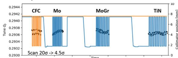
Figure 3: The raw tune data shows a clear reduction of the tune shift with the new coatings with respect to the CFC. A significant tune drift during the measurement can also be seen. The orange line depicts the position of the standard CFC secondary collimator, the blue line – the 3-stripe collimator. Black dots show individual tune measurements.
