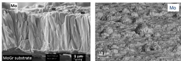
Figure 6: Mo coating is not uniform: it has a column-like fine structure (left) and inhomogeneities up to 10  $\mu\text{m}$  on its surface (right) SEM image results [15].
