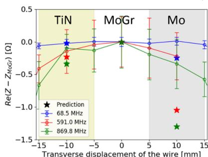
Figure 7: The measured difference in the real part of the longitudinal impedance suggests a higher than expected resistivity of the Mo stripe. Resonant wire measurement, performed in a test stand prior to the installation of the three-stripe collimator in LHC.
