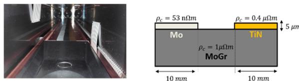
Figure 2: The prototype collimator has two 10 mm wide low resistivity (Mo and TiN) stripes on a MoGr substrate. Left - photo of the collimator assembly; right - schematic drawing of the collimator jaw.
