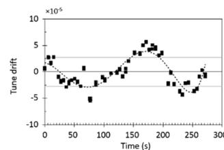
Figure 4: A slow tune jitter with a  $\sim 100$  s period and an rms spread of  $\pm 2 \times 10^{-5}$  (thin grey lines) is observed during the ADT excitation tune measurements.
