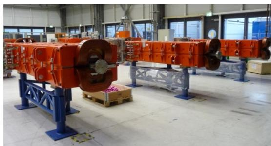
Figure 3: Dipole magnets (built by NIIIEFA) with installed vacuum chambers (built by BINP) shipped to GSI.
