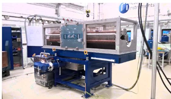
Figure 2: First of Series (FOS) SIS100 acceleration cavity at factory acceptance test.
