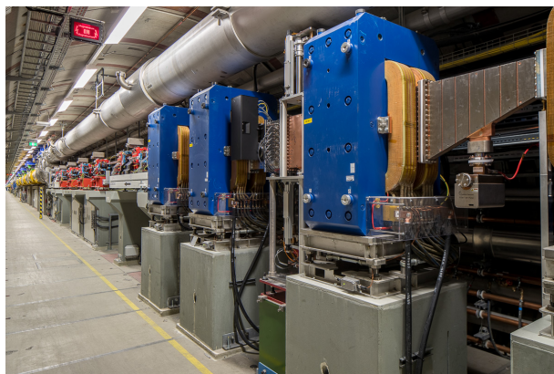
Figure 1: The first bunch compressor and parts of the European XFEL's main linac in the background on the left hand side. The grey tube in the upper part of the picture is a helium transfer line feeding the cryostats of the cold linac.
