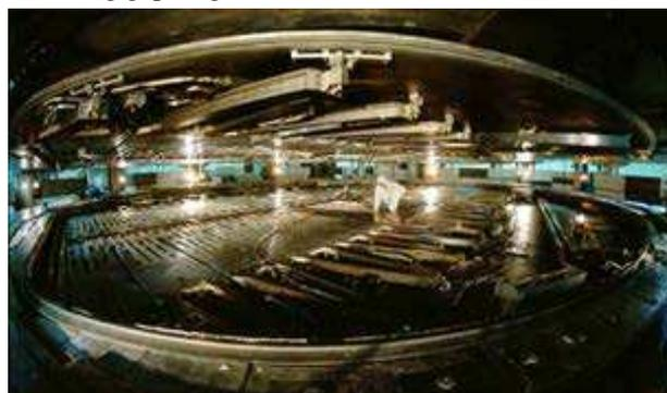
Figure 3: Inside the vacuum tank with lid raised– showing the 80 rf resonator segments fixed to the base and lid, and (right) one of the long 4.2 K cryopanel.
