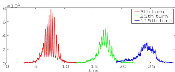
Figure 4: Longitudinal beam profile at the 5th (red), 25th (green), 115th (blue) turns in the DR.
