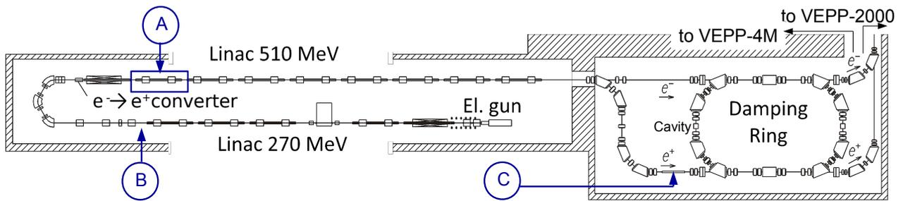
Figure 3: VEPP-5 IC layout with expected improvements of the machine: a - 3 additional quadrupoles for stronger e+ beam focusing, b - additional RF structure to increase e- beam energy, c - debuncher to reduce energy spread of the e+ beam.
