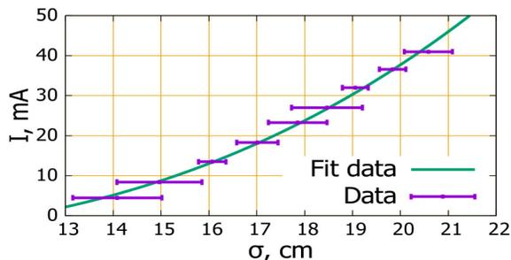
Figure 5: Longitudinal beam size vs beam current, data were taken at  $U_{RF} = 9.4$  kV.
