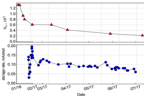
Figure 2: Beam charge emitted from the electron gun (top), single shot storage rate of the positrons in the DR (bottom) as function of operating period of the gun cathode in the 2016/2017 season.
