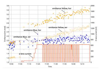
Figure 2: Blue and Yellow rms emittances as measured by the IPMs (left scale), and electron lens current (right scale). The detailed time function of the electron lens current is shown in Figure 1.
