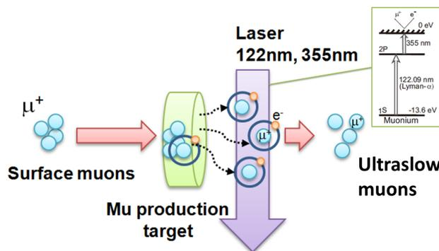
Figure 1: Principle of ultra-slow muon production.
