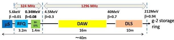
Figure 5: Configuration of the muon linac.
