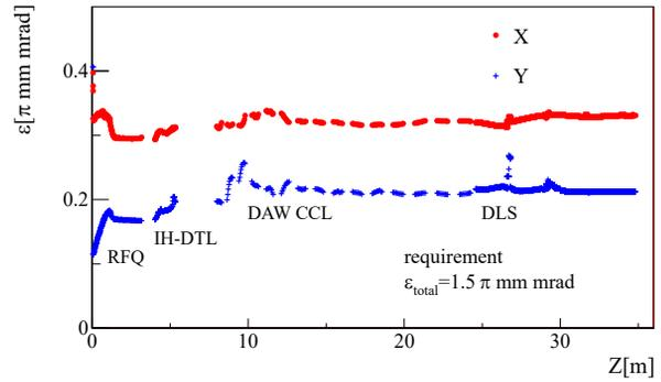
Figure 9: Emittance evolution from the RFQ entrance to the linac exit.
