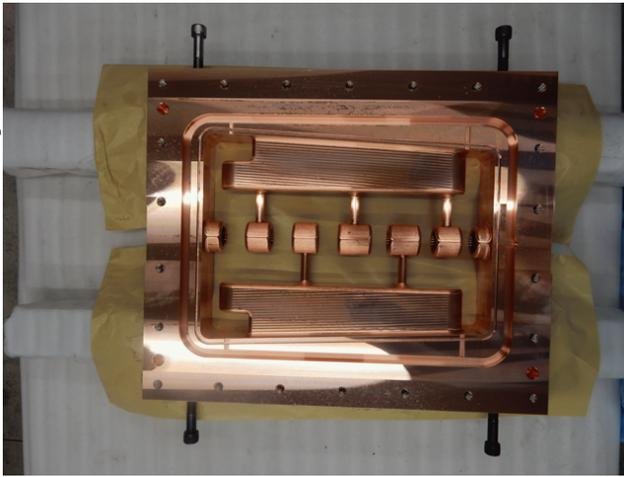
Figure 8: Center plate of 6-cell prototype IH DTL.
