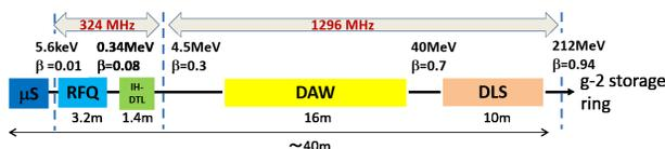
Figure 5: Configuration of the muon linac.
