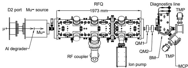
Figure 11: Schematic drawing of the setup of the muon acceleration experiment.
