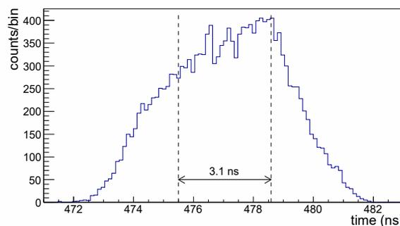
Figure 7: Time structure of the  $\mu^+$  beam at the RFQ entrance.
