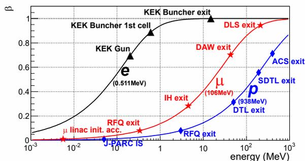
Figure 4: Comparison of the velocity evolution with energy for electron (KEKB injector [11]), proton (J-PARC H- linac [12]) and muon linacs.
