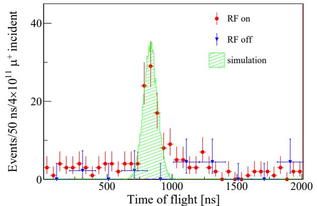
Figure 13: TOF spectra with RF on and off. The clear peak of the RF on spectrum at 830 ns corresponds to the accelerated  $\text{Mu}^-$ 's. A simulated TOF spectrum of the accelerated  $\text{Mu}^-$ 's is also plotted.
