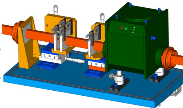
Figure 4: Sketch of cylinder lens setup for beam transport of ArF ionization laser. On the right side the laser safety shutter is shown.
