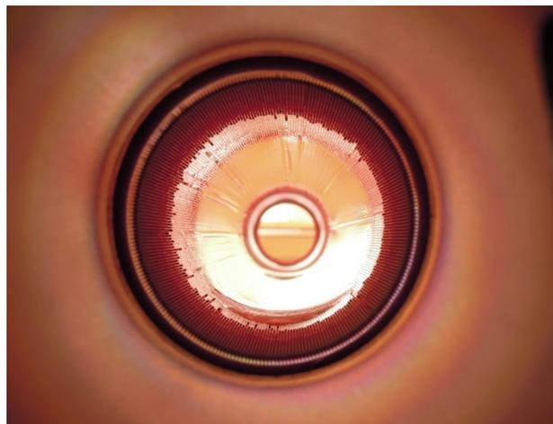
Figure 2: View into the test heat pipe oven with grooves. The hot part in the middle is evenly covered with lithium.
