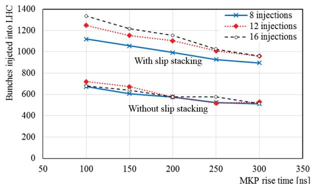
Figure 1: Possible numbers of bunches injected into LHC as a function of the SPS injection kicker rise time for 8, 12 and 16 injections into the SPS per cycle. The beneficial effect of shorter kicker rise time and slip-stacking are clear.
