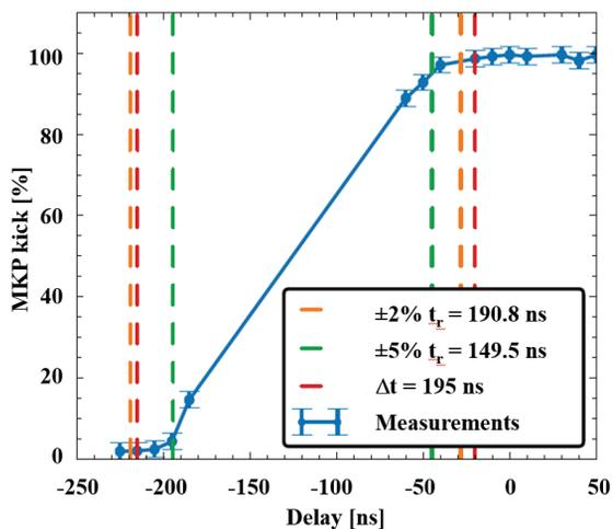
Figure 3: Measured MKP kicker waveform using magnets 1-3 at 49 kV for ion injection. A rise time of just below 150 ns is achieved (5-95%).
