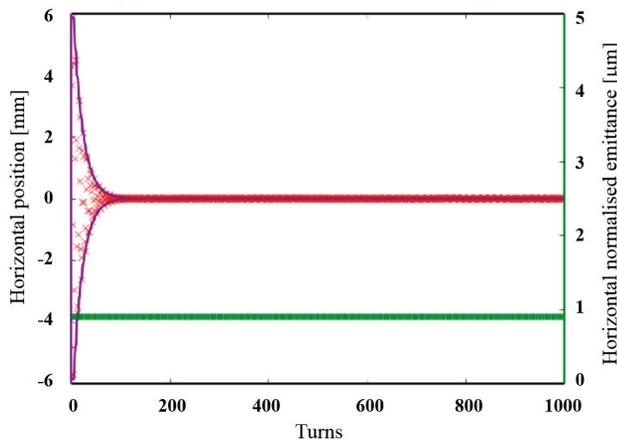
Figure 4: Simulated damping of injection oscillation of 6 mm in presence of amplitude detuning with 1/e damping time of 20 turns. No measurable blow-up is expected.
