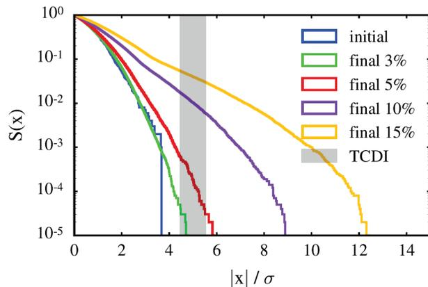
Figure 6: Simulated bunch distribution after injection damping of the initial truncated Gaussian, for different SPS residual injection kick errors. The TCDI jaw at  $5 \pm 0.5 \sigma$  is shown.
