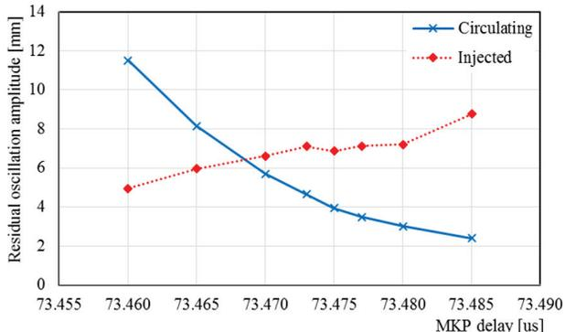
Figure 2: Measured residual oscillations on injected and circulating trailing ion bunches for 150 ns MKP rise time. For the optimum settings both bunches are kicked about 6 mm with respect to the orbit.
