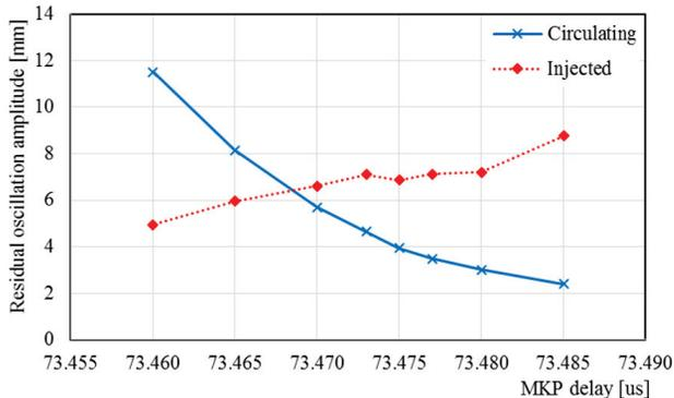
Figure 2: Measured residual oscillations on injected and circulating trailing ion bunches for 150 ns MKP rise time. For the optimum settings both bunches are kicked about 6 mm with respect to the orbit.
