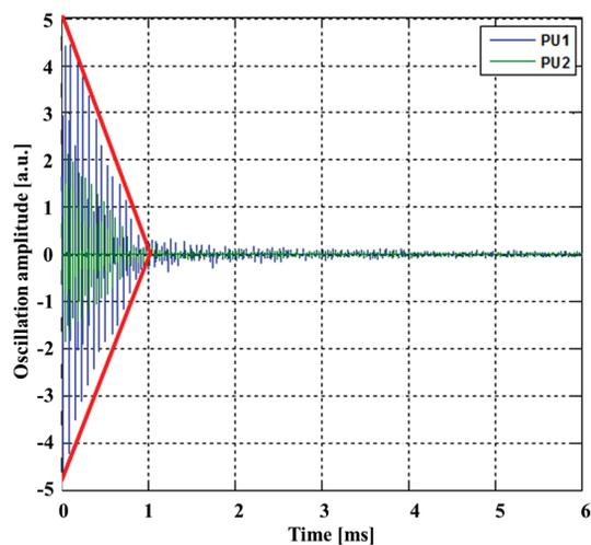
Figure 5: Measured damping of injection oscillation of 6 mm, with oscillations completely damped within 1 ms (40 turns). The  $1/e$  damping time is about 24 turns.
